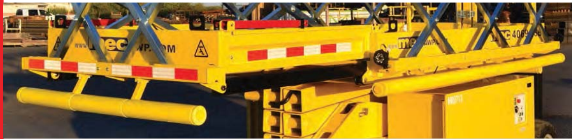
APPB (Aircraft Padded Protection Bumpers) with or without cut-out Sensors
