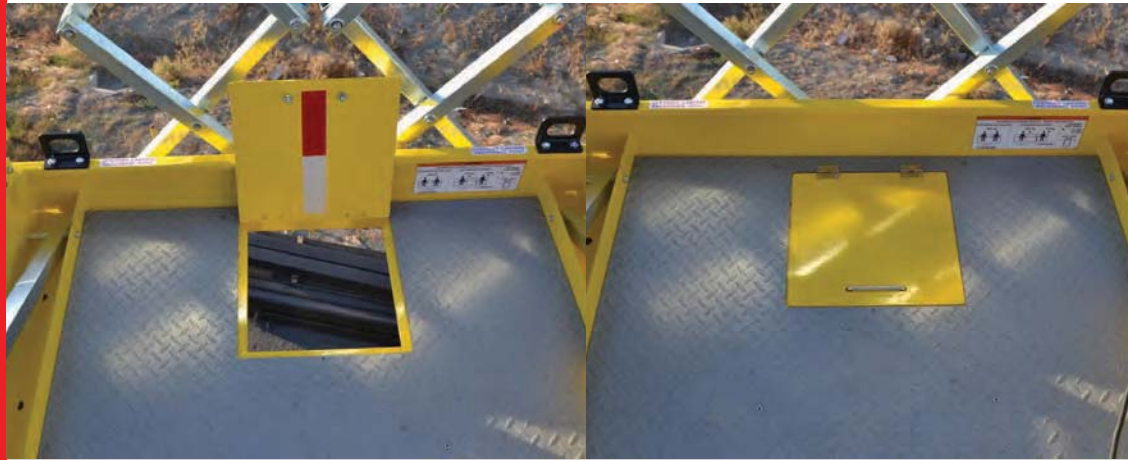
On board access door designed for Over-Wing maintenance
