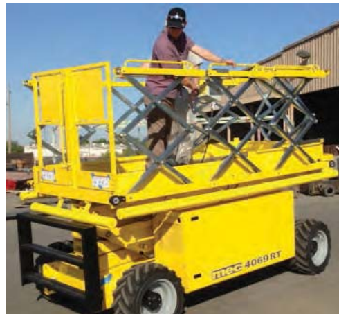
Low Entry of 1.3 m (51 in) and Dual rear Entry gates
