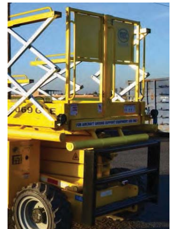
Low Entry of 1.3 m (51 in) and Dual rear Entry gates
